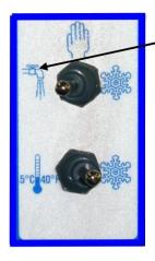
Cleaning Operation - The drive motor will run in the faucet position to allow a stirring action of the rinse water while cleaning.
